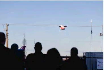
DDC's Sparrow drone is used for delivering small parcels at a max range of 20km and payload of approximately 4kg.
